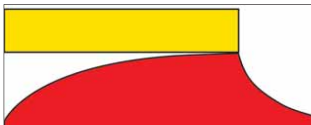
Figure 1. A schematic of the temperature rise associated with the application of continuous-wave laser energy. The yellow bar represents the duration of the laser pulse, and the red represents the rise and fall of the temperature of the treated tissues.
