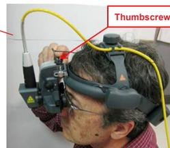
6. Adjust pupillary distance (PD) between the oculars for image fusion. While observing through both oculars, the user should be able to comfortably read printed material held at or near the retinal image plane (approximately 370 - 430 mm or 14.6 - 16.9 inches from the headset)
