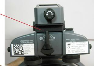
2. Select intermediate illumination spot using the Aperture Control Lever
