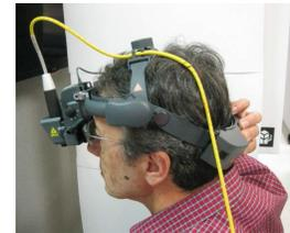
5. Adjust up/down and forward/back-ward location of the slots of LIO viewing assembly using thumbscrew and secure position with the thumbscrew
