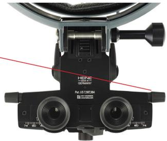
7. Using the condenser lens and vertical aiming beam knob located beneath the dust cover assembly, focus and position the aiming beam in the center of the illumination field already projected on the patient's forehead.
