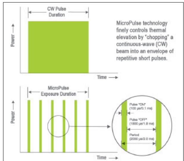
Figure 1. The mechanism of action of MicroPulse technology.
